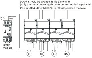
For frame A, terminal + (-) is connected to the terminal + (-) of the brake module. For frame B, C and D, terminal +/B1 (-) is connected to the terminal + (-) of the brake module.
