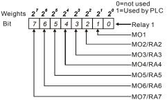
For example: when Pr.03.09 is set to 3 (decimal) = 00000011 (binary) that indicates Relay1 and MO1 are used by PLC. (Pr.03.09= 2<sup>0</sup>+2<sup>1</sup>=3)
