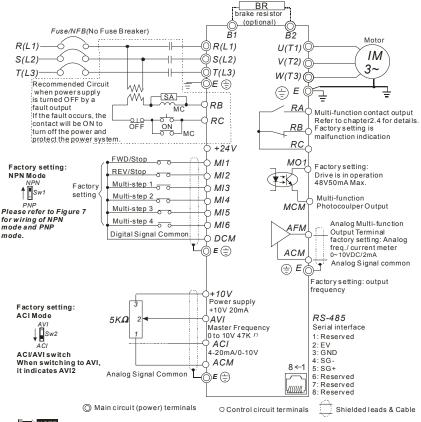
For VFD-E-T series, the braking resistor can be used by connecting terminals (B1 and B2) directly. But it can't connect DC-BUS in parallel.
