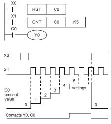
32-bit high-speed addition/subtraction counter C235:
