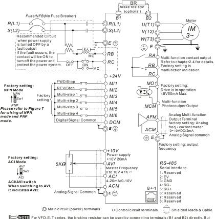
TE For VFD-E-T series, the braking resistor can be used by connecting terminals (B1 and B2) directly. But it can't connect DC-BUS in parallel.
